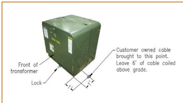
Front side of pad-mounted transformer with lock
