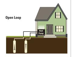
Ground source heat pumps (GSHPs) are electrically powered systems that tap the stored energy of the greatest solar collector in existence: the earth. These systems use the earth's relatively constant temperature to provide heating, cooling and hot water for homes.
